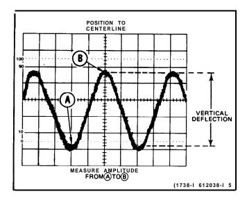
Figure 11. Peak-to-peak waveform voltage.
