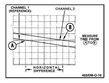
Figure 19. High-resolution phase difference.
