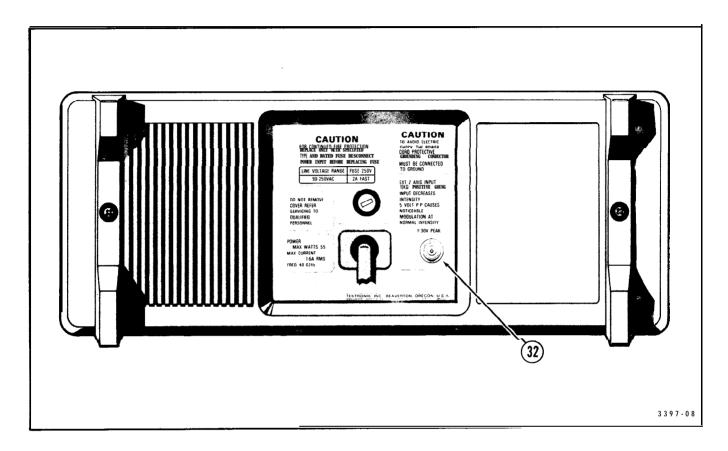
Figure 7. Rear-panel connector.
