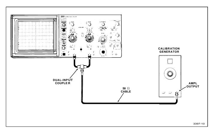
Figure 9. Initial setup for instrument familiarization procedure.
