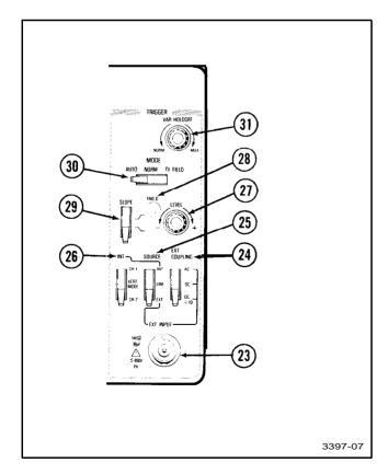
Figure 6. Trigger controls, connector, and indicator.
