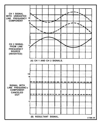
Figure 14. Common-mode rejection.
