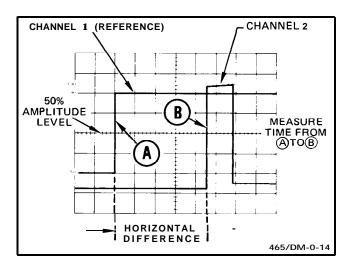
Figure 17. Time difference between two time-related pulses.
