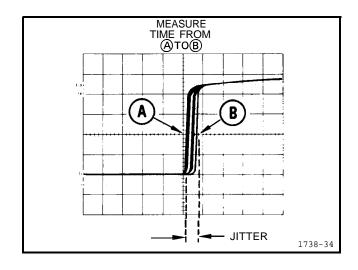
Figure 21. Pulse jitter.
