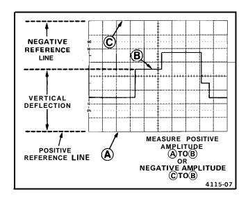
Figure 12. Instantaneous voltage measurement.
