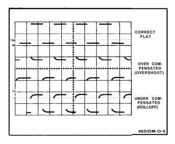
Figure 10. Probe compensation.
