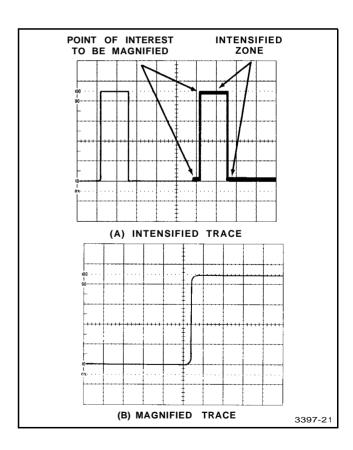
Figure 20. Delayed-sweep magnification.
