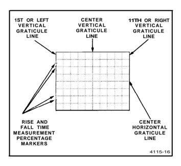
Figure 8. Graticule measurement markings.
