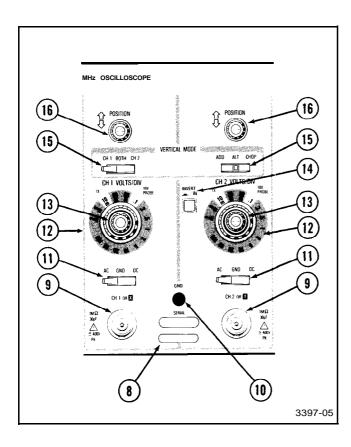
Figure 4. Vertical controls and connectors.
